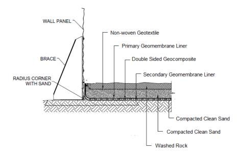
Once a geomembrane has been installed either within a containment system or to line an earthen pit the geomembrane is relatively safe. However, if there is further construction activity on the site that requires the geomembrane to come into contact with crews or machinery. It is a relatively simple process for our crews to add or modify the liner to allow for expansion or modifications to the containment.
